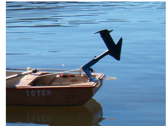
Motor in ready to lower position
