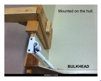
On this particular boat, the placement of the mount was reasonably close to a bulkhead, which provides side panel stiffness, and as such, the mount will have little twisting effect on the hull. Placed further away from the bulkhead may require the application of an inside panel stiffener.
