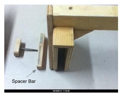
The finished mount with the spacer bar and locking bolt.
