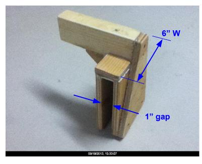
The design of the Mount intentionally places the Motor close to the side of the Hull. This produces the smallest moment arm. which translates to less downward side force. The shift of battery location easily offsets this force, and produces a balanced boat.
