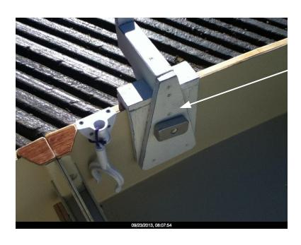
The Mount secured to the side of the hull.
