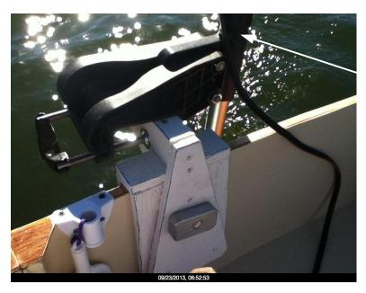
Under full power, and no noticeable flex of the hull. It's a good idea to slightly tighten the locking collar on the motor shaft, to prevent the motor from wandering, and allowing hand's free cruising..
