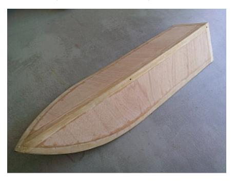
The total cost of building these sponsons (2) is about \$20, if you have left over materials from building the boat. If this is an only build, the cost should be less than \$40. These sponsons add an additional 24 inches to the beam of the TOTER 2 hull, providing an all weather experience.
