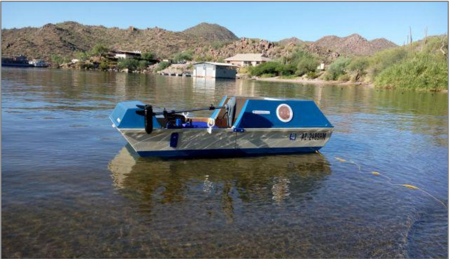
This photo shows the 30 pound thrust (PT) trolling motor mounted on the starboard rear side of the hull. This is the best location as far as ease of use is concerned, if you are right handed, as the throttle is within easy reach of the pilot seated center in the hull. For larger motors there is a rear mount option, but a 30 PT motor is all the boat really needs, it's lower in cost and it also conserves battery power.
