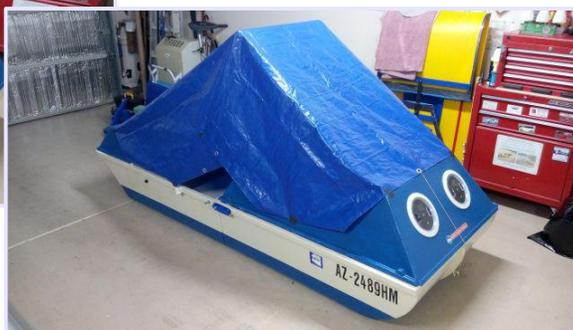
that encloses the hull completely, yet folds away under the forward seats when not in use.
