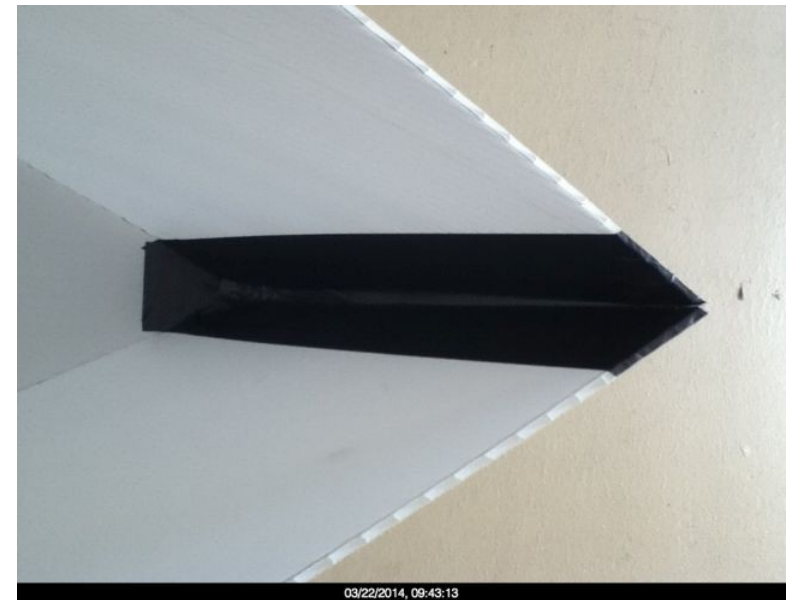
Inside bow triple taped seam.
