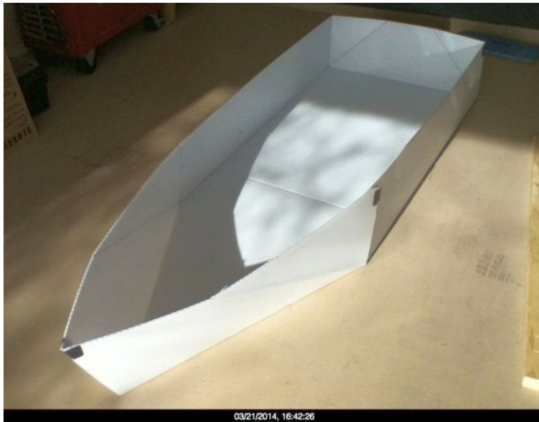
Hull temporarily taped together, checking folds.
