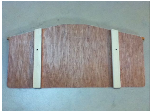
Transom (back) with 1x2 vertical supports spaced 16" apart
