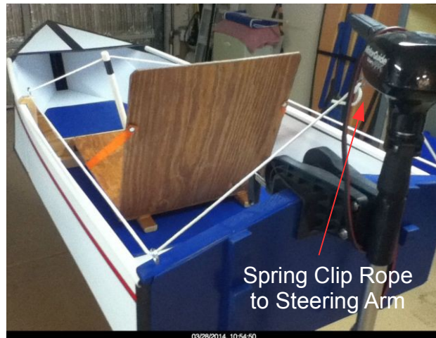
1/4" Nylon Rope, from Motor to Tiller
