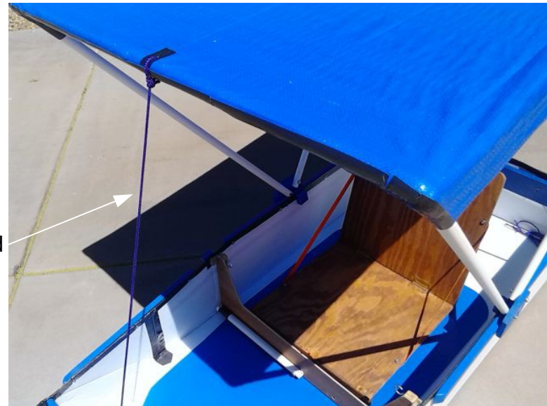
Canopy top taped to frame
