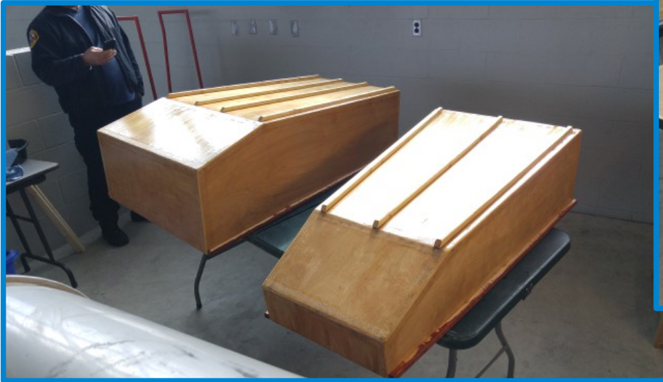
Forward and rear modules after waterproofing.
