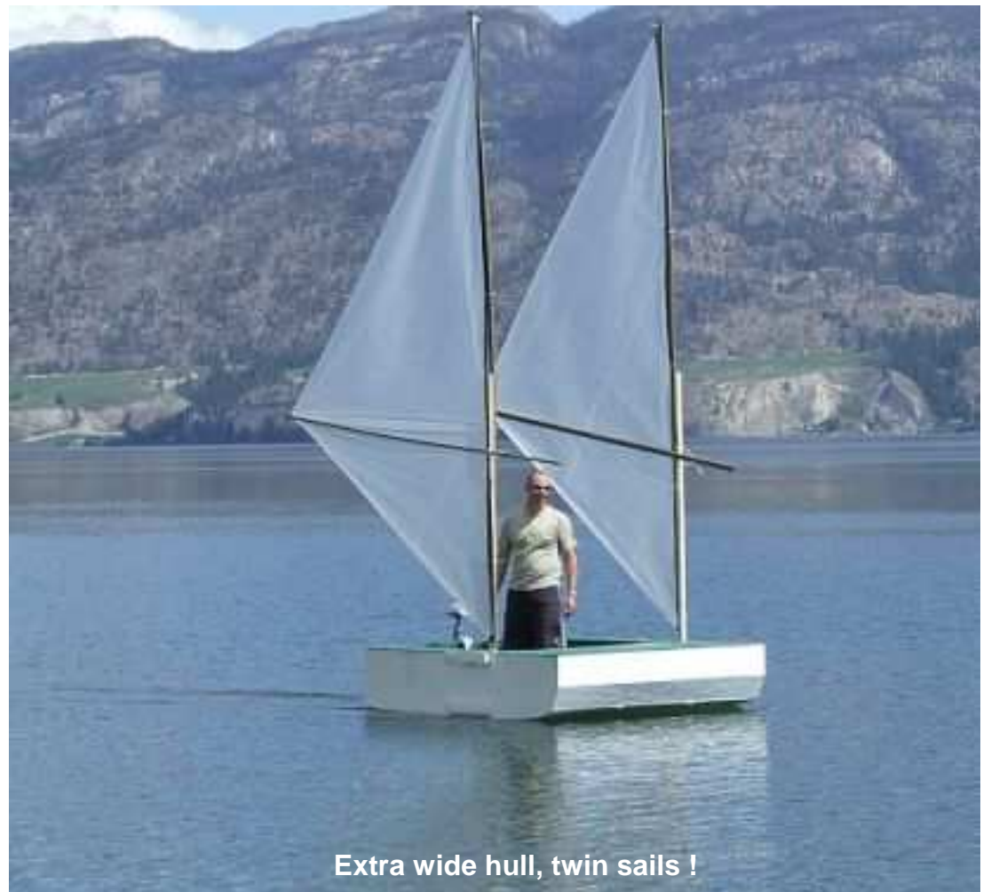
Open Construction with Expanded Sail Area
