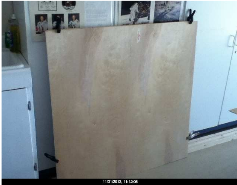
Plywood 4 x 4 sheets clamped together to keep them from warping prior to cutting.
