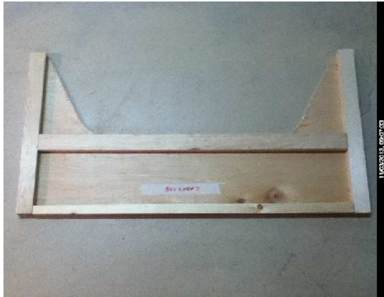
Bulkhead brad stapled and laying on flat surface to cure. Weigh down if necessary to keep flat..
