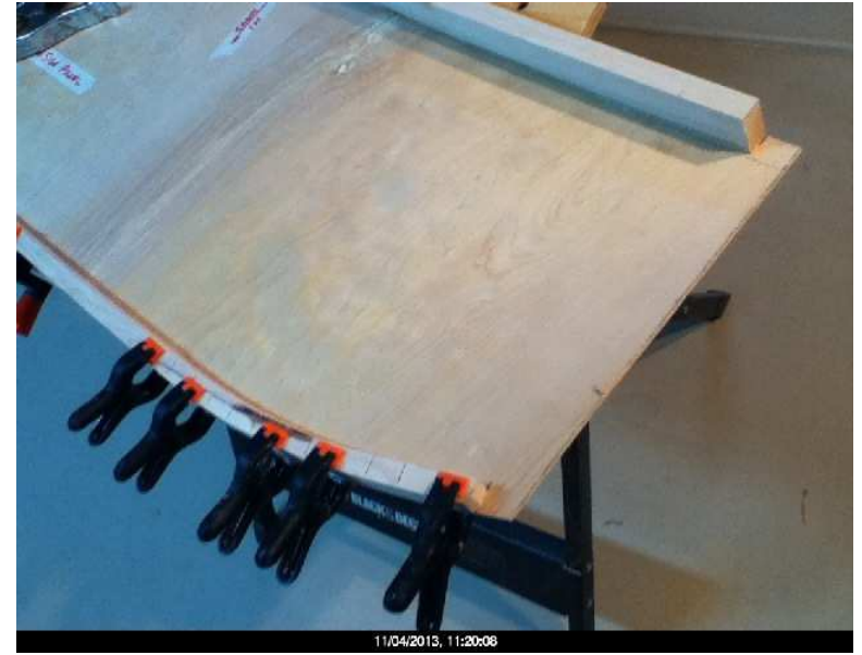
Bottom stringer glued, clamped and stapled in place
