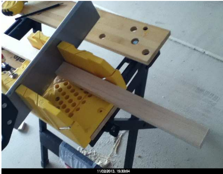
Cutting a side support using a miter box.
