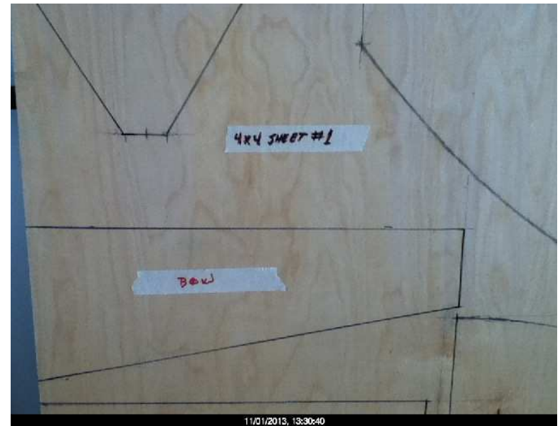
Marked Panels using a Sharpie. Notice the bow curve, and the masking tape panel markers.
