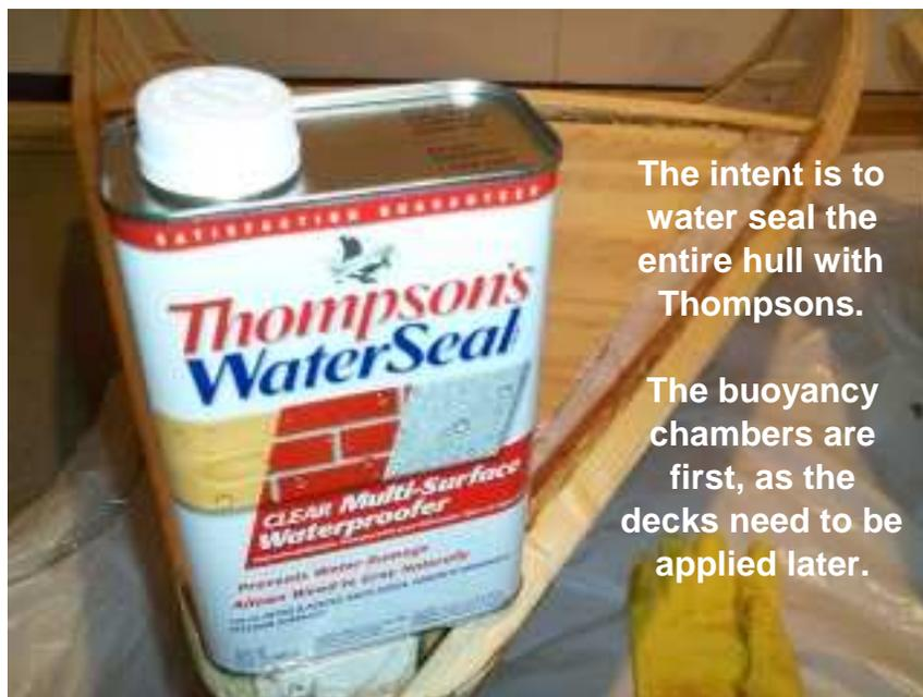
The intent is to water seal the entire hull with Thompsons.
