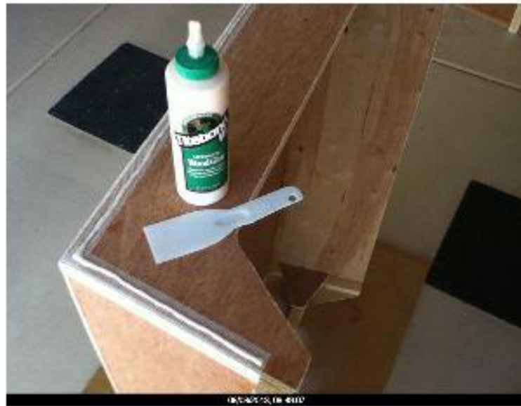
Typical glue bead size
