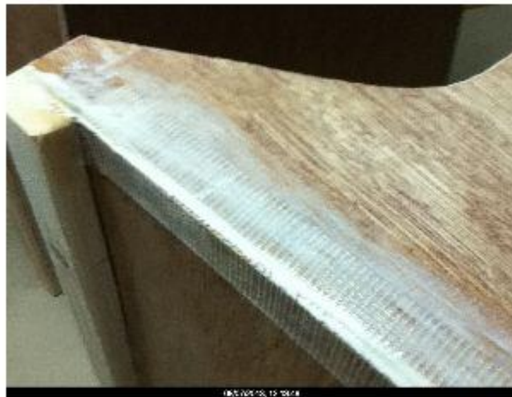
Finished taped edge
