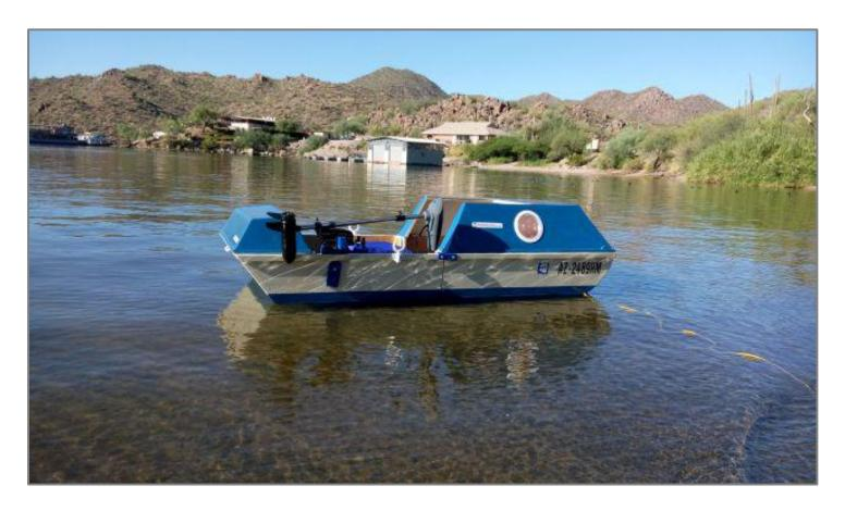
This photo shows the 30 pound thrust (PT) trolling motor mounted on the starboard rear side of the hull. This is the best location as far as ease of use is concerned, if you are right handed, as the throttle is within easy reach of the pilot seated center in the hull. For larger motors there is a rear mount option, but a 30 PT motor is all the boat really needs, it's lower in cost and it also conserves battery power.
