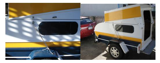
• Do not use the small black plastic deck cleats for hold down. These are only for light deck lines when tied to a jetty or pontoon.
